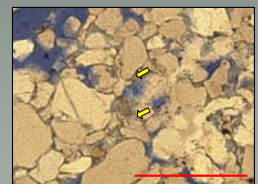
Figure 6: Photomicrograph of Mount Cap Fm glauconitic (arrows) quartz sandstone. Sample 06LP-21-14, plane polarized light. Red scale bar = 0.5 mm.
