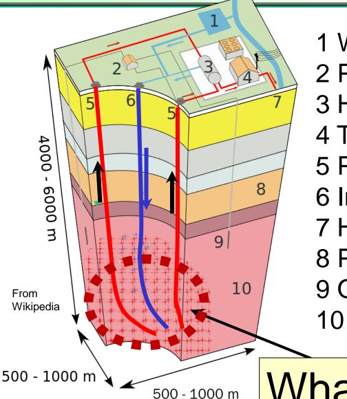
1 Water lagoon 2 Pump house 3 Heat exchanger 4 Turbine hall 5 Production well 6 Injection well 7 Hot H<sub>2</sub>O to district heating 8 Porous sediments 9 Observation well 10 Crystalline bedrock
