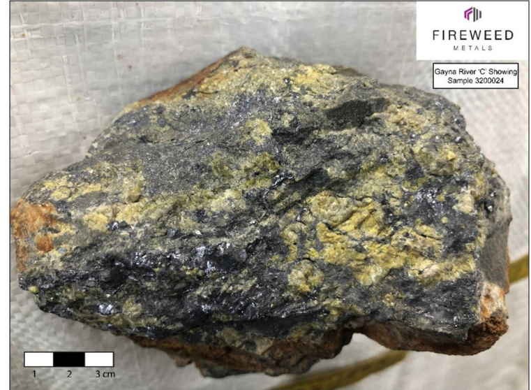
Gayna Project Rock Sample with Massive Galena-Sphalerite
