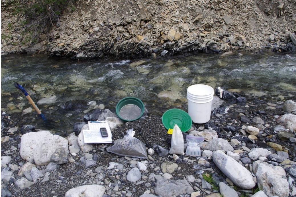
Figure 8. Examples of typical tools used during bulk sampling for HMC concentrates, silt and water sampling. A sample suite is shown, including a 12-kilogram sample contained in the polyethylene bag to the left of the 20-litre plastic white pail. The sieve and plastic gold pan used during the wet sieving are sitting to the right of the short-handled spade used for excavating the material. A silt sample is contained in a Hubco sack (white with yellow tag in front of gold pan). Water samples are in 125 ml Nalgene bottles within the zip-lock bags. Also shown are Garmin GPS to identify and record sample locations and a checklist form to record observations on waterproof paper.
