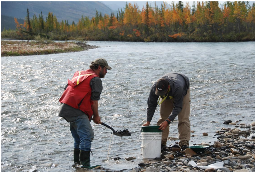
Figure 7. HMC Sample collection including sieving and washing the sandy material from river gravels into a plastic bag lining the inside of the pail.
