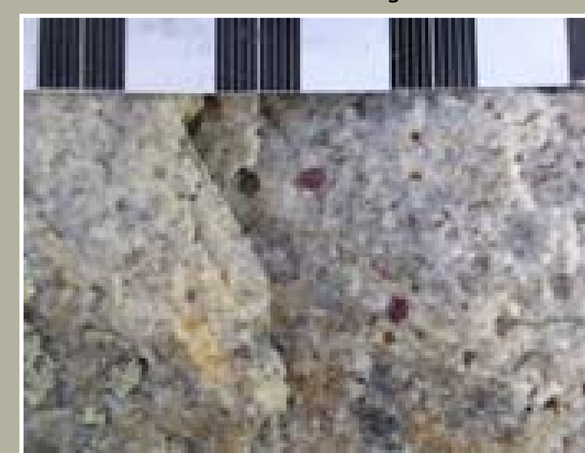
Accessory minerals in the monzogranite include rare garnet, tourmaline, sillimanite and apatite. Shown above are pink garnets in muscovite-bearing pegmatitic monzogranite.
